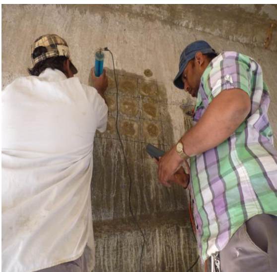
Half cell Potentiometer test
