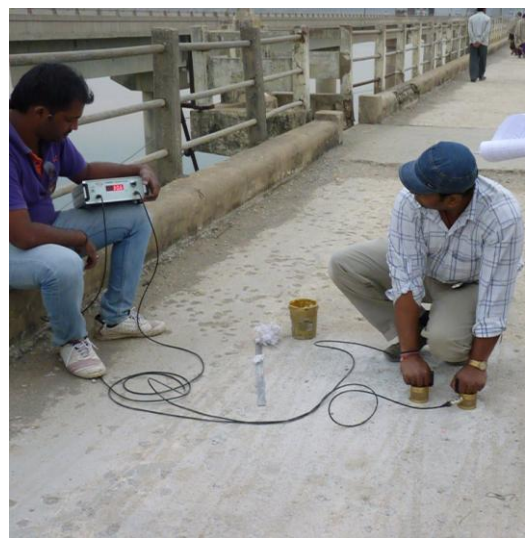
Ultra Pulse Velocity test by indirect method
